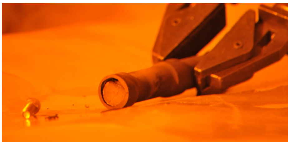
First 1-step UC x target after irradiation with 20 \mu A of protons at ISAC. Target and target material show no signs of ageing. Picture taken in the ISAC south hot cell.
